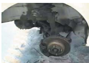
NSF suspension assembly is pushed to the back of the wheel arch, resulting in damage to the wing
