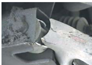
NSF steering rack arm, bent by the impact when this car hit the kerb
